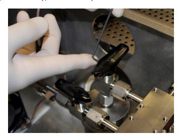
b. Using an adjustable wrench and a 3/4" wrench, turn (counter clockwise) the VCR fitting connecting the bottle valve with the manifold.
