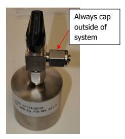
6. Install bottles with a new SS ¼" VCR fitting using the same procedure outlined above but turning clockwise to tighten the connection between the bottle and the manifold.
